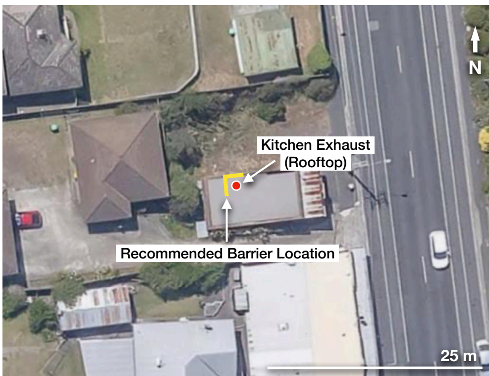
FIGURE 7.1: RECOMMENDED KITCHEN EXHAUST BARRIER LOCATION
