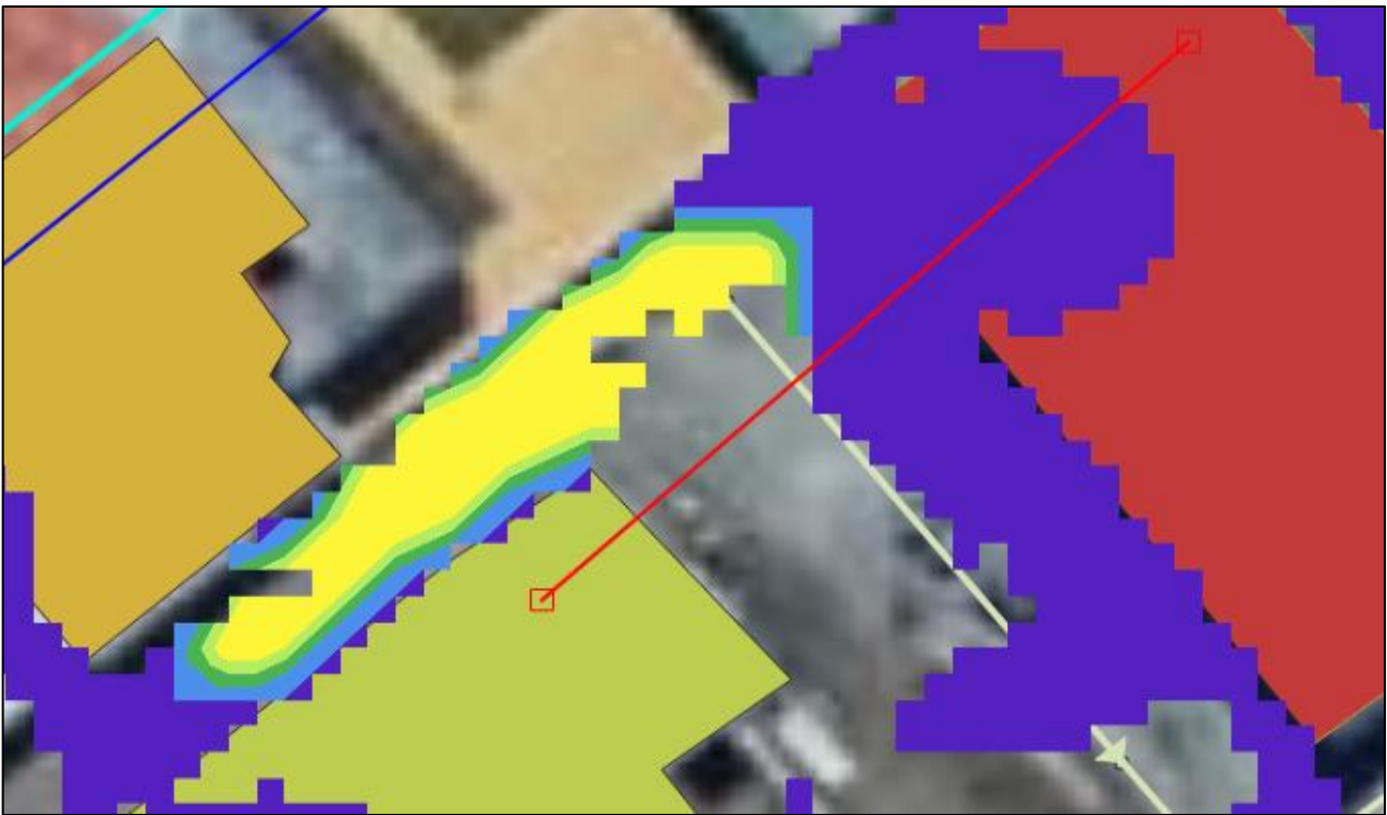
Figure 17 – Zoom-in of hazard mapping – 1% AEP, 540 min, TP10 – RCP8.5
